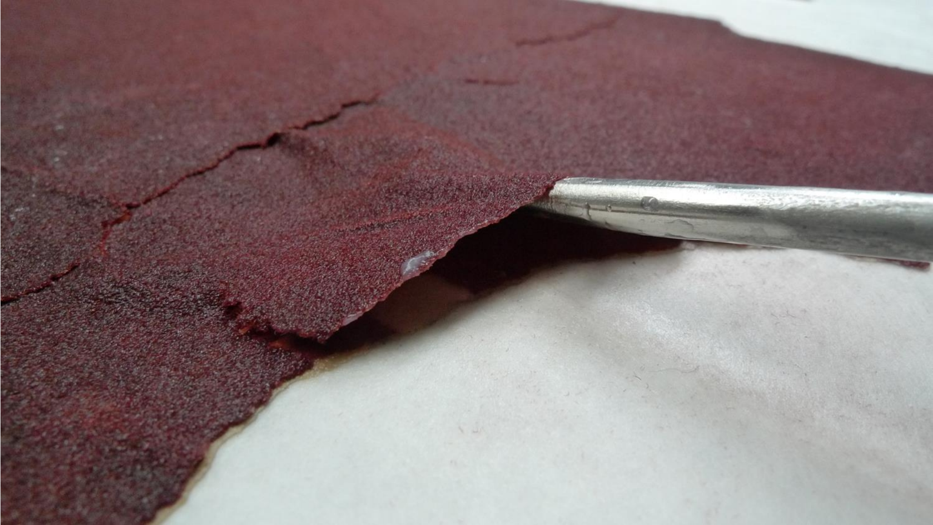
Not just cellulose fibers but also mounting glue can expand during wet treatment
